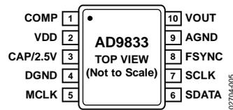
Figure 5. Pin Configuration
