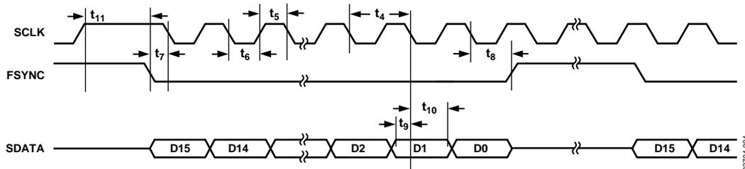
Figure 4. Serial Timing
