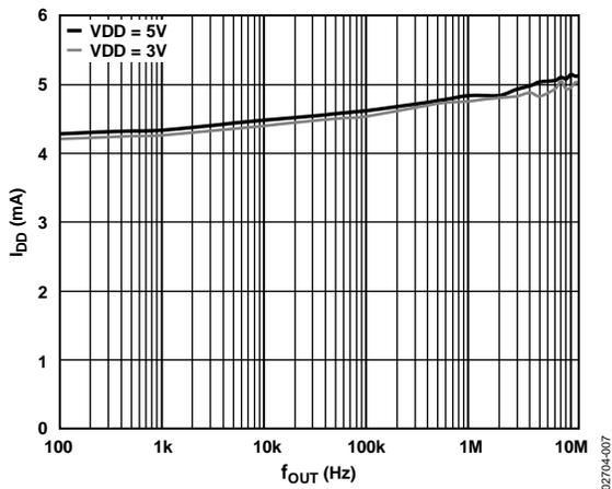
Figure 7. Typical  $I_{DD}$  vs.  $f_{OUT}$  for  $f_{MCLK} = 25$  MHz
