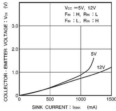
Fig.8 Output saturated voltage vs. sink current (I)
