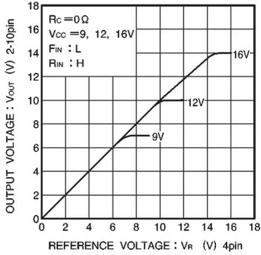
Fig.13 Output voltage vs. reference voltage ( II )
