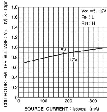
Fig.11 Output saturated voltage vs. source current (II)
