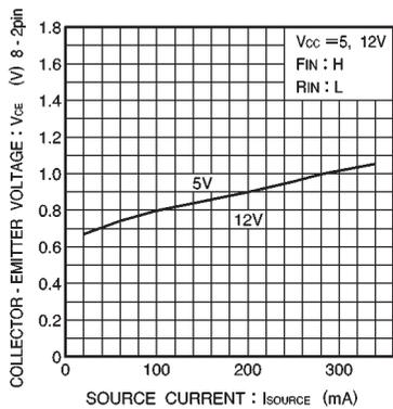
Fig.10 Output saturated voltage vs. source current (I)
